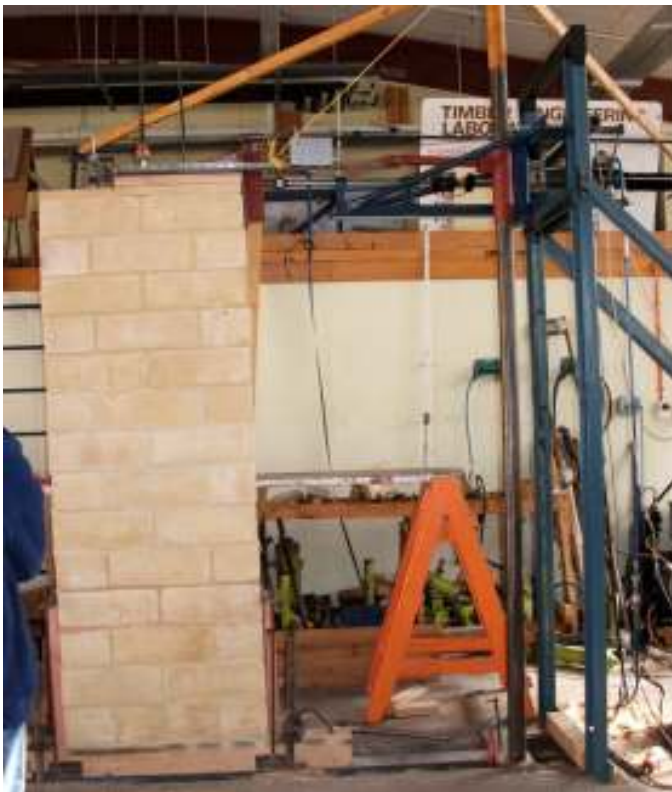
Photo 3: Shows 880mm wall at 55mm top plate deflection
