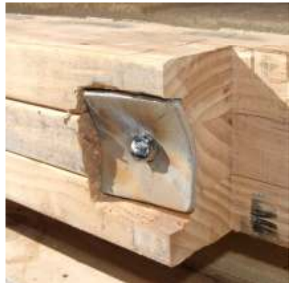
Photo 2: Shows 80x80 washers after racking to 55mm
