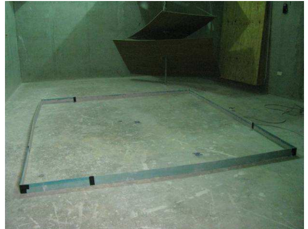
Figure 2: Fibre cement frame left in the reverberation room as part of the empty room.
