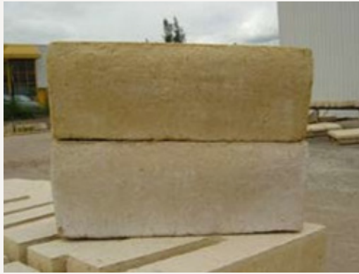
Block with efflorescence cleaned with Enviro Pacific efflorescence remover.
