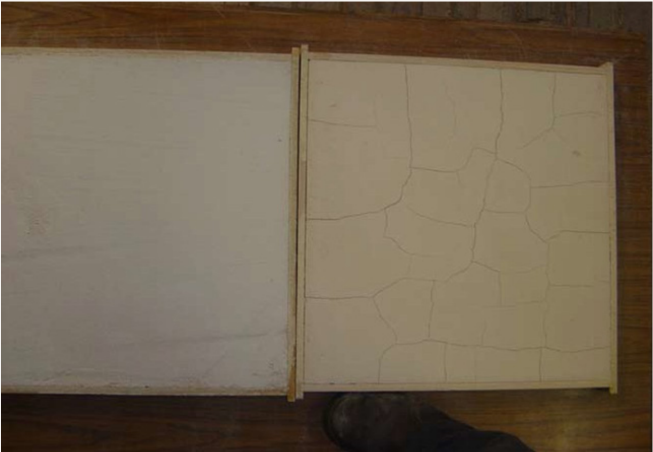
Testing mortar mixes with cracking appearing on the right
